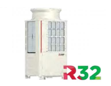
Mitsubishi's City Multi R2 series offers high efficiency heat recovery. Global Warming Potential from refrigerant use is limited through use of R32 refrigerant and a wet heat distribution system, which limits refrigerant volume compared to systems that use refrigerant for heat distribution throughout the building. © Mitsubishi
