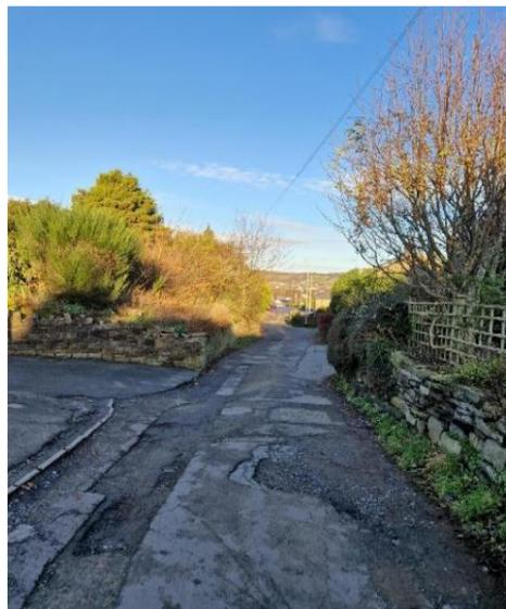
*Photo 8: Privately maintained section of Colders Lane for private carriage access to residential properties. Uneven surface with several layers of tarmac.*
