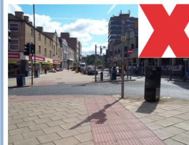
Stud tactile pavers or brass studs are required at pedestrian crossings and corduroy at level changes. These should be designed sensitively and sensibly. Studs should be raised enough to serve their purpose but not overtly proud. Where possible tactile units should be made of matching materials to the surroundings.
