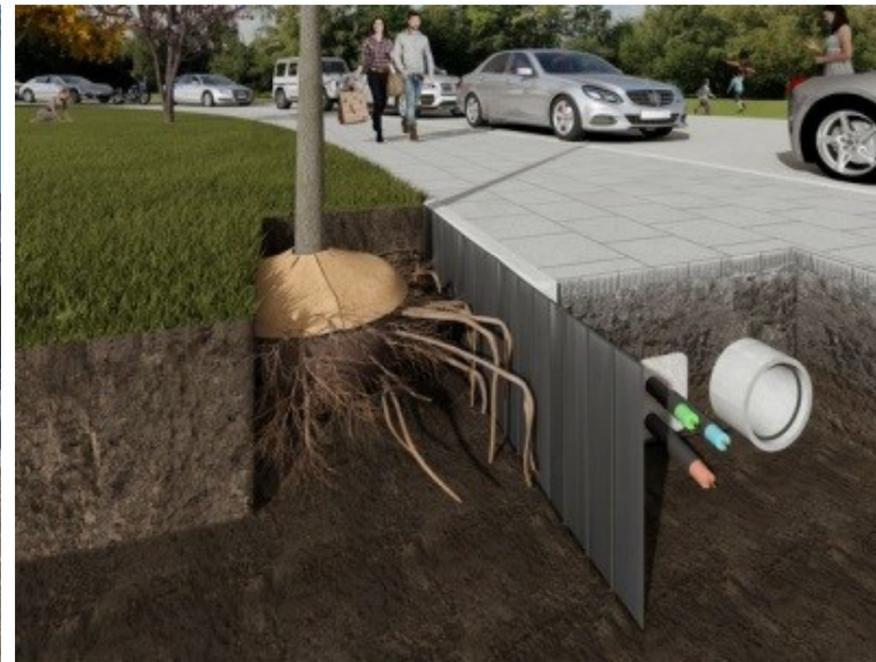
Urban tree planting usually requires the use of special load bearing underground structures which prevent upheave of pavements and compaction around tree roots. They can also prevent tree root penetration into service pipes.
